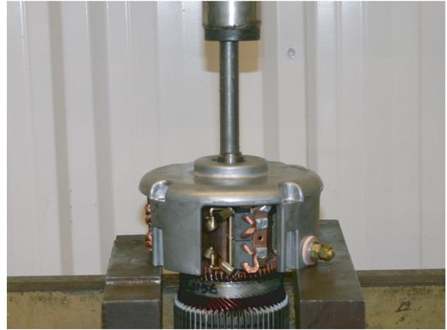
Figure 27-7 Armature Removal
