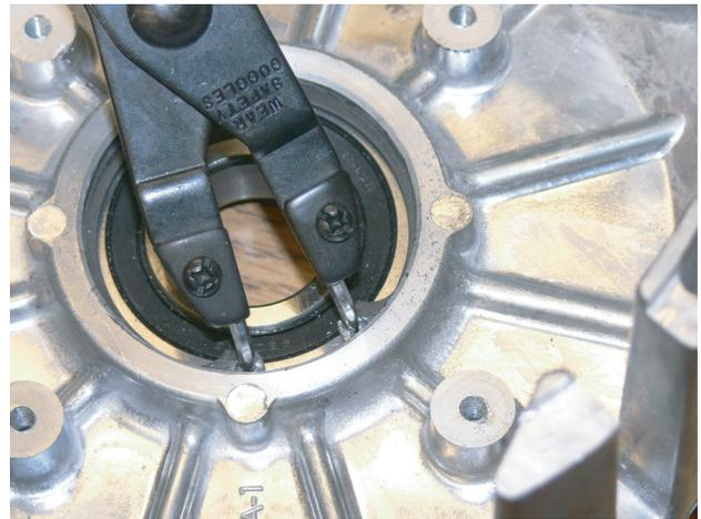
Figure 27-9 Retaining Ring Removal
