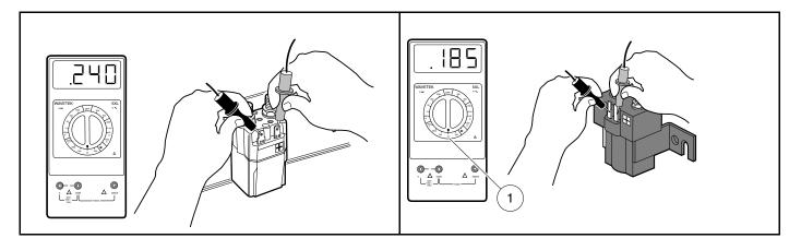
Figure 14-8 Activating Coil Test – Factory-installed Solenoid
