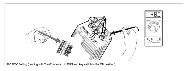
Figure 12-20 Pin 10 Test
