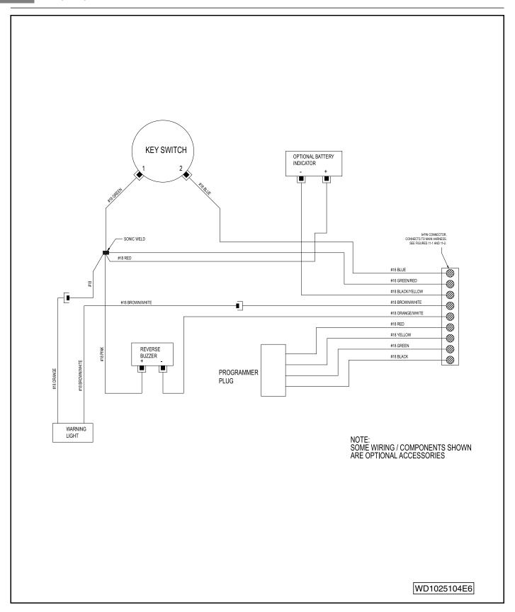
Figure 12-5 Precedent Electric Vehicle Instrument Panel Wiring Diagram
