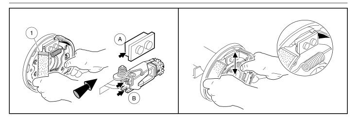
Figure 6-15 Install Leading Shoe
