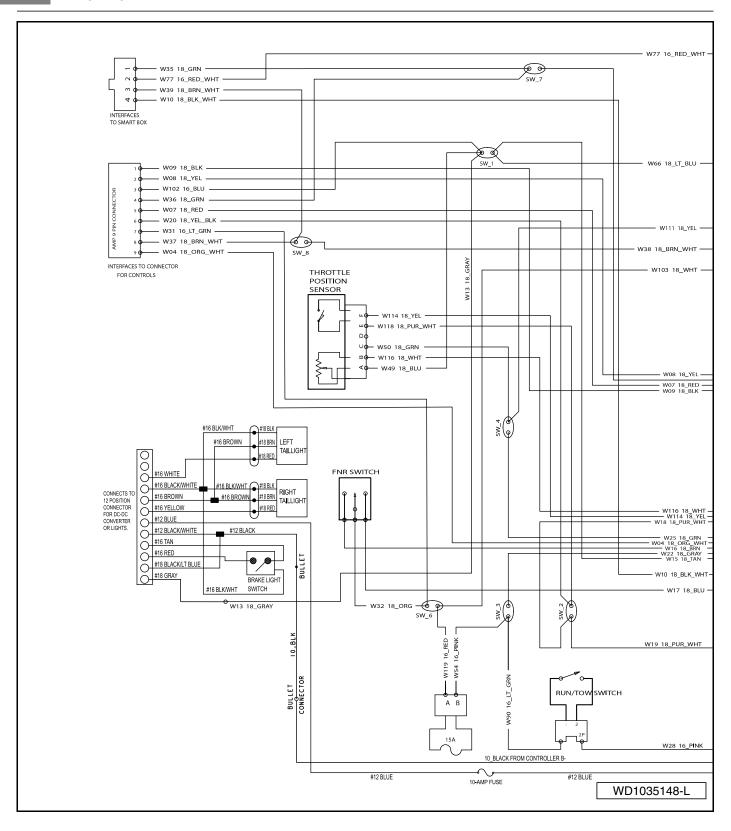
Figure 13-4 Wiring Diagram – Excel System with TPS
