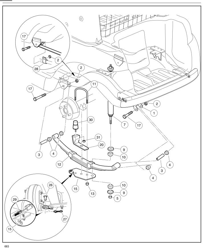
Figure 9-4 Rear Suspension Assembly and Mounting (Four-Passenger Vehicles)
