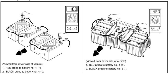
Figure 14-6 Battery Voltage Test – Style B Battery Configuration
