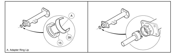
Figure 21-3 Axle Seal and Adapter Ring
