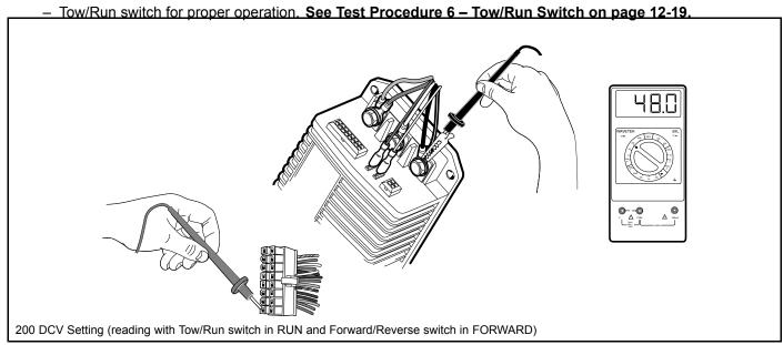
Figure 12-18 Pins 8 and 16 Test
