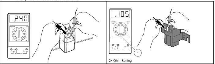
237 Figure 11-8 Activating Coil Test - Factory-installed Šolenoid
