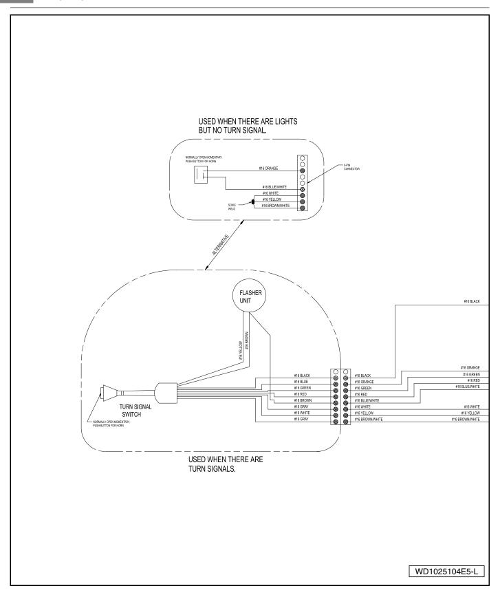
Figure 14-2 Precedent Electric Vehicle Accessory Wiring Diagram
