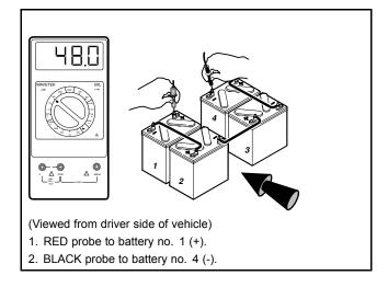
Figure 12-6 Battery Voltage Test – Style A Battery Configuration
