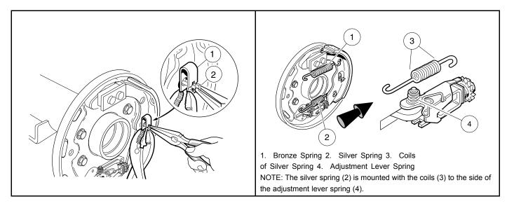
Figure 6-13 Install Trailing Shoe Retainer Clip
