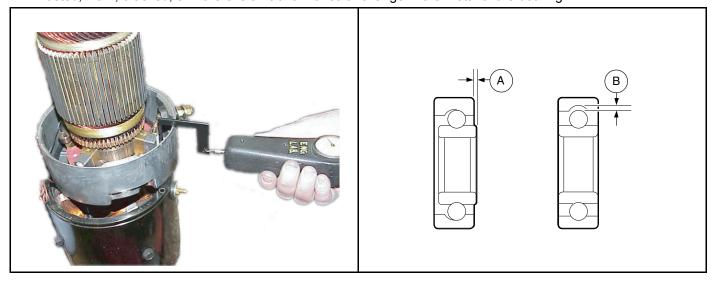
756 Figure 20-13 Brush Spring Tension Test
