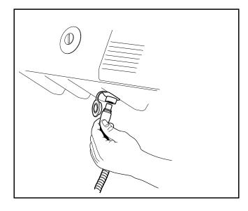
Figure 22-1 IQDM Port Under Instrument Panel
