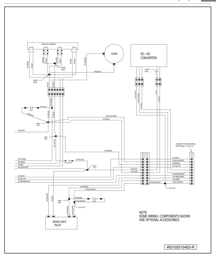
Figure 12-4 Precedent Electric Vehicle Accessory Wiring Diagram (Continued)
