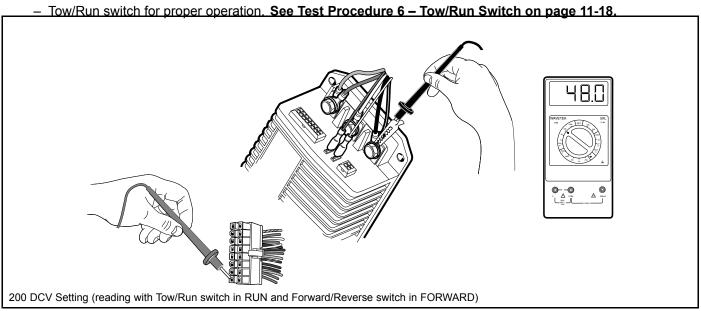
Figure 11-14 Pins 8 and 16 Test
