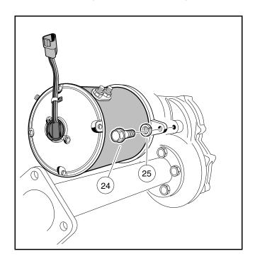
Figure 21-12 Motor Positioning Bolt – EJ4–4001 and 5BC59JBS6390 Motors Only
