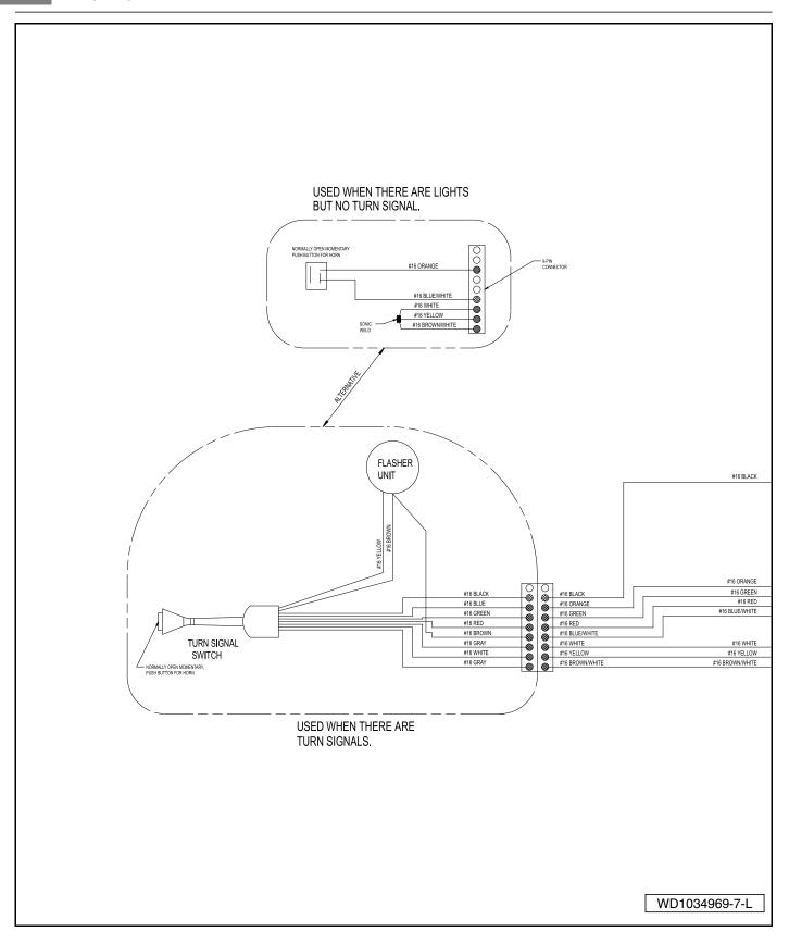
Figure 11-3 Precedent Electric Vehicle Accessory Wiring Diagram
