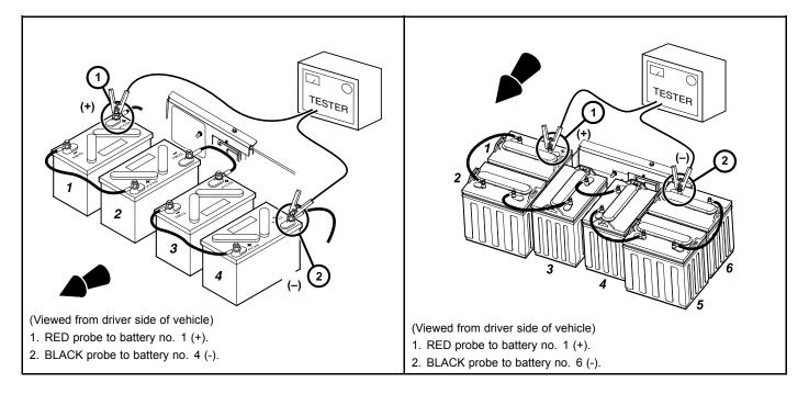
Figure 13-10 Battery Discharge Test – 4 x 12 Volt Battery Figure 13-11 Battery Discharge Test – 6 x 8 Volt Battery Configuration
