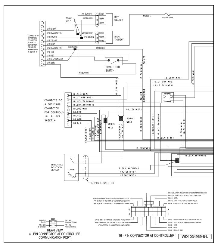
Figure 11-1 Wiring Diagram - IQ System with TPS
