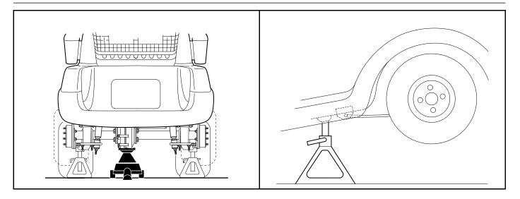
729 Figure 20-1 Lift Vehicle with Floor Jack
