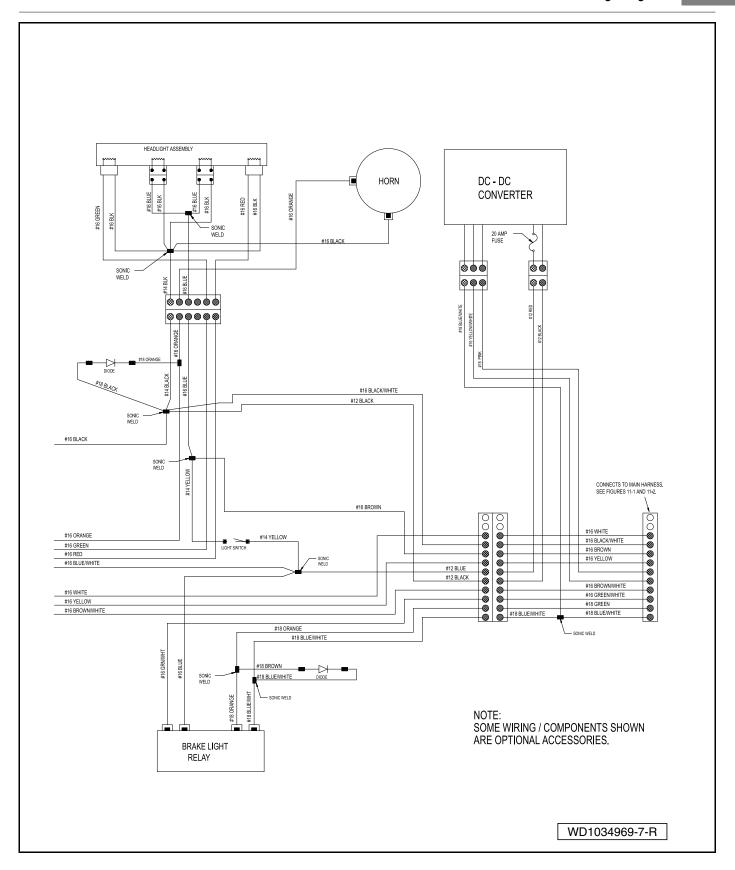
Figure 11-4 Precedent Electric Vehicle Accessory Wiring Diagram (Continued)
