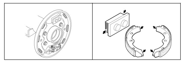
Figure 6-9 Apply Grease On Bosses
