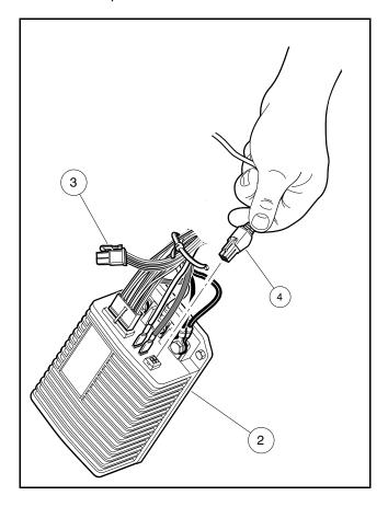
Figure 16-9 IQDM Connector On Speed Controller
