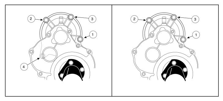
Figure 20-24 EJ4–4001 Motor Mounting Bolts and Tightening Sequence
