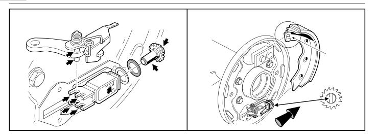
Figure 6-11 Apply Grease To Brake Adjuster
