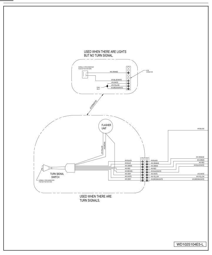
Figure 12-3 Precedent Electric Vehicle Accessory Wiring Diagram
