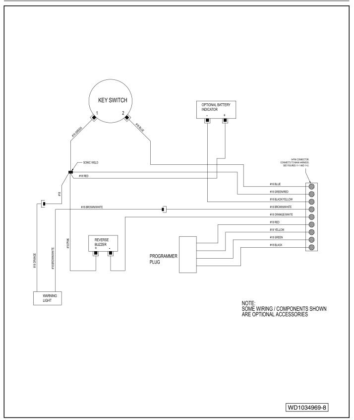
Figure 13-1 Precedent Electric Vehicle Instrument Panel Wiring Diagram
