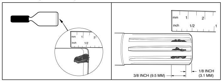
Figure 20-20 Grease on Putty Knife
