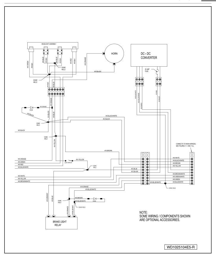
Figure 14-3 Precedent Electric Vehicle Accessory Wiring Diagram (Continued)
