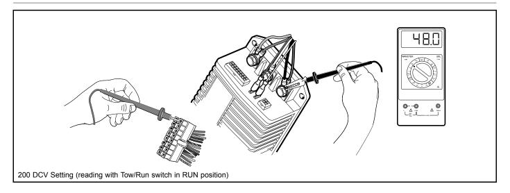
Figure 11-15 Pin 9 Test
