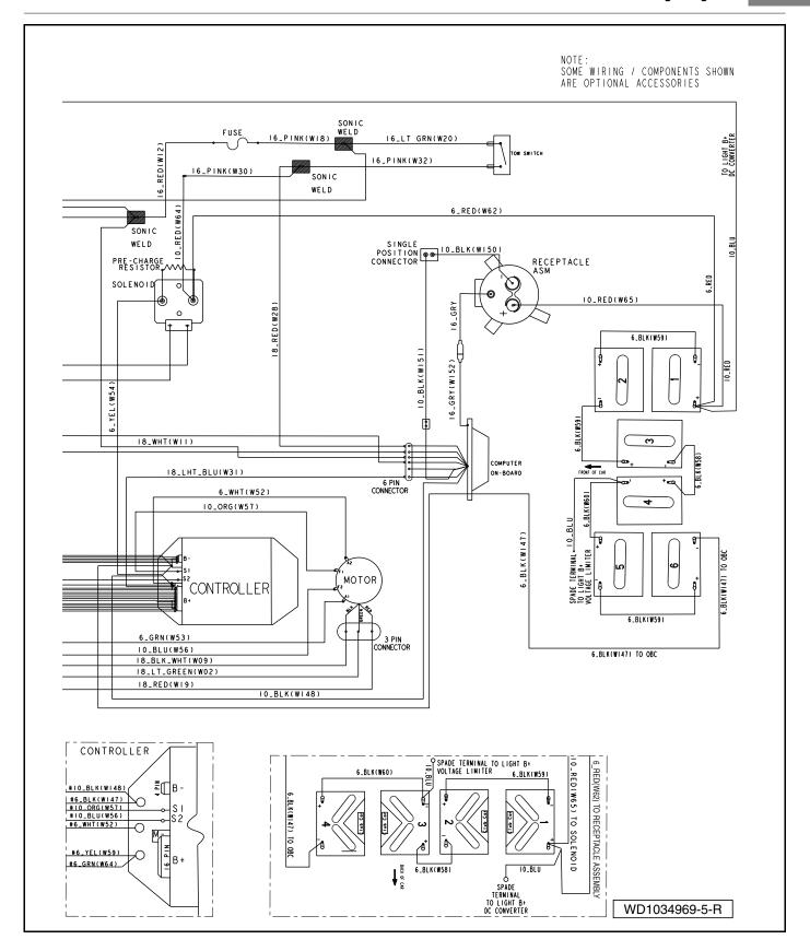
Figure 11-2 Wiring Diagram – IQ System with TPS (Continued)
