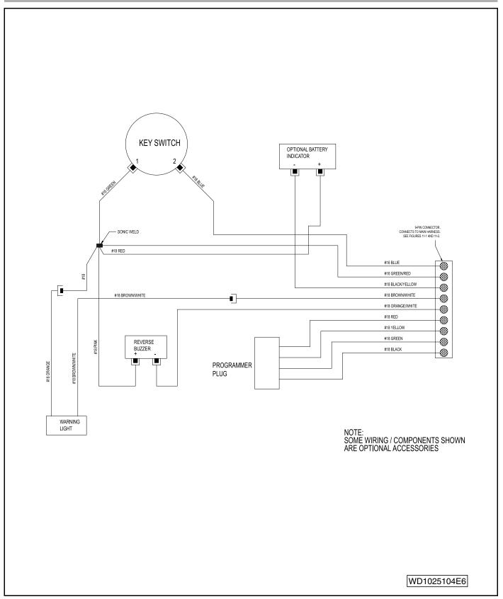
Figure 14-1 Precedent Electric Vehicle Instrument Panel Wiring Diagram
