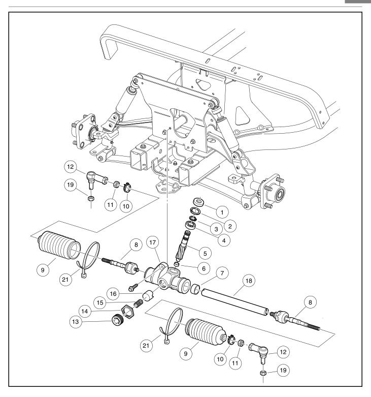
Figure 7-5 Steering Gear
