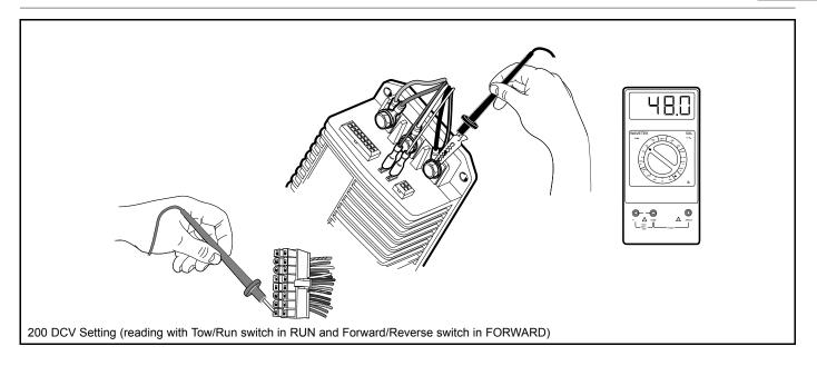
Figure 14-16 Pins 8 and 16 Test
