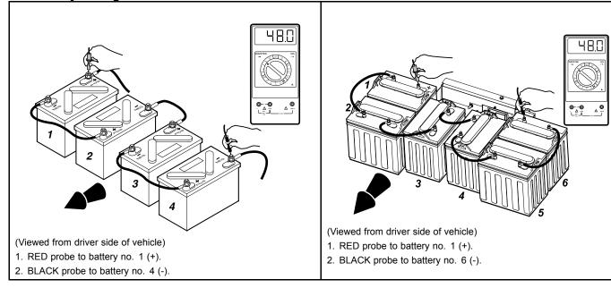
Figure 13-6 Battery Voltage Test – 4 x 12 Volt Battery Configuration
