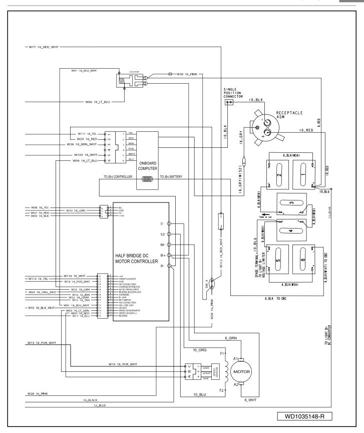
Figure 13-5 Wiring Diagram – Excel System with TPS (Continued)
