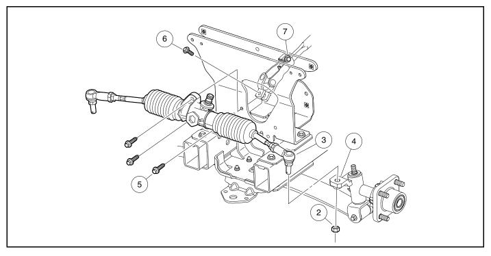
Figure 7-4 Rack and Pinion Removal
