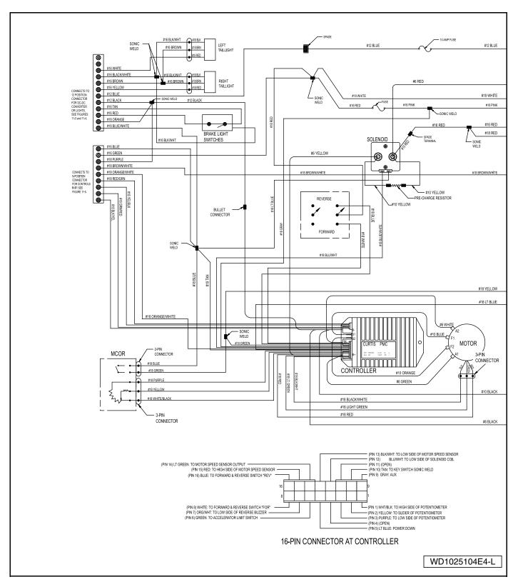
Figure 12-1 Wiring Diagram – IQ System with MCOR
