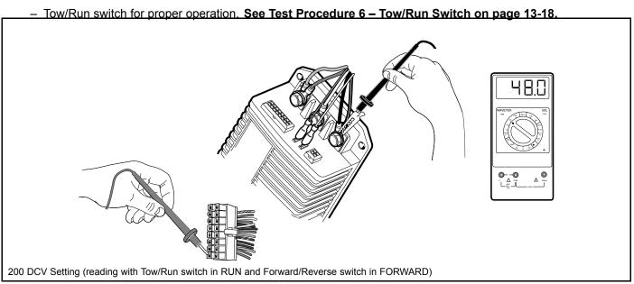
Figure 13-14 Pins 8 and 16 Test
