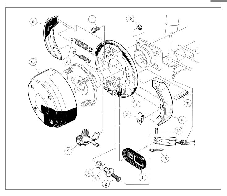
Figure 6-4 Self-adjusting Wheel Brake Assembly
