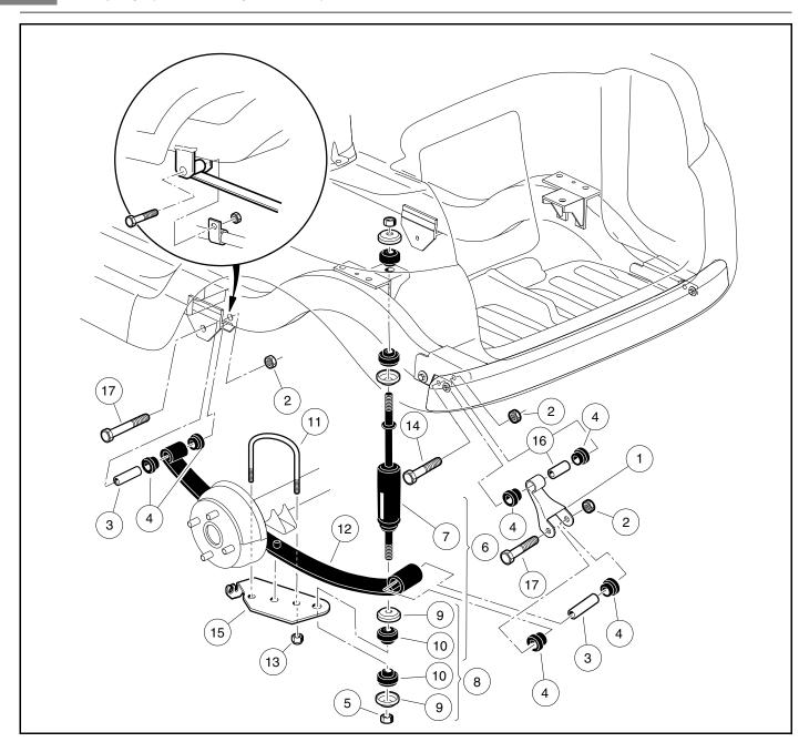
Figure 9-3 Rear Suspension Assembly and Mounting (Two-Passenger Vehicles)
