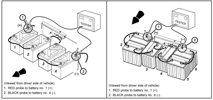
2500-30100-10410 Figure 12-12 Battery Discharge Test - Style B Battery Configuration
