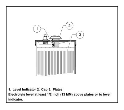
17 Figure 18-8 Battery Electrolyte Level
