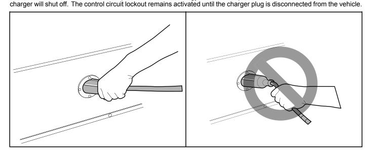
Figure 18-9 Correct Insertion of Charger DC Plug
