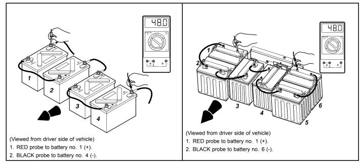
Figure 11-6 Battery Voltage Test – 4 x 12 Volt Battery Configuration
