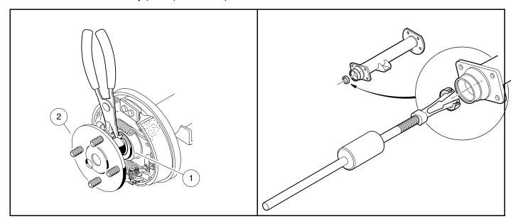
762 Figure 21-1 Remove Internal Retaining Ring
