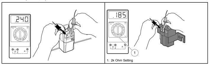
2377 Activating Coil Test - Factory-installed Figure 13-8 Solenoid
