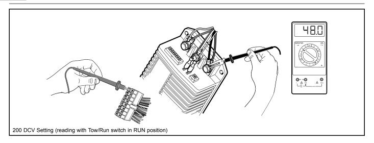
Figure 12-19 Pin 9 Test
