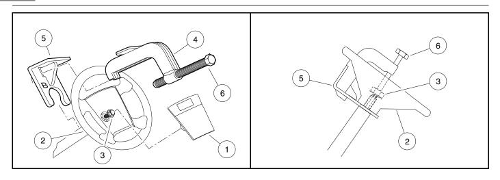
Figure 7-1 Steering Wheel Removal
