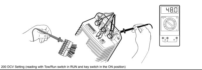
Figure 11-16 Pin 10 Test
