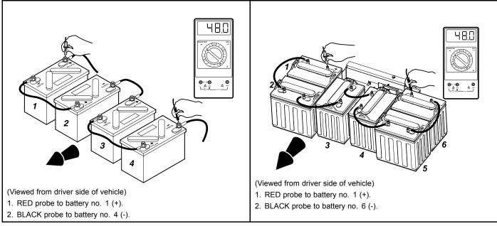
Figure 12-7 Battery Voltage Test – Style B Battery Configuration
