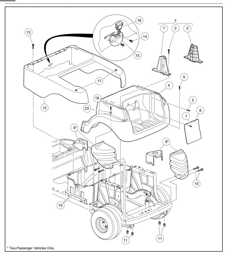
Figure 4-8 Rear Body Components
