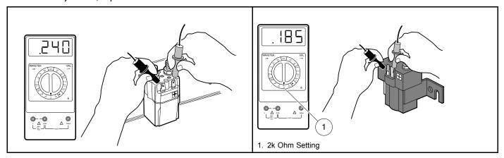
Figure 12-9 Activating Coil Test – Factory-installed Solenoid
