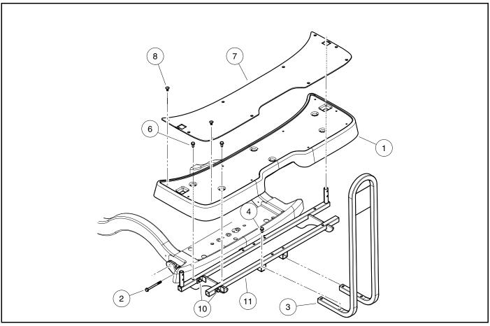
Figure 4-11 Foot Deck (Four-Passenger Vehicles)
