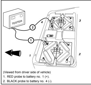
2500-30100-10409 **Figure 12-11** Battery Discharge Test - Style A Battery Configuration
