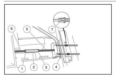
Figure 6-20 Loosen Brake Cables
