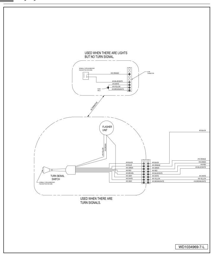
Figure 13-2 Precedent Electric Vehicle Accessory Wiring Diagram
