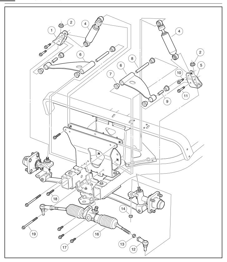
Figure 7-19 Upper Front Suspension Assembly
